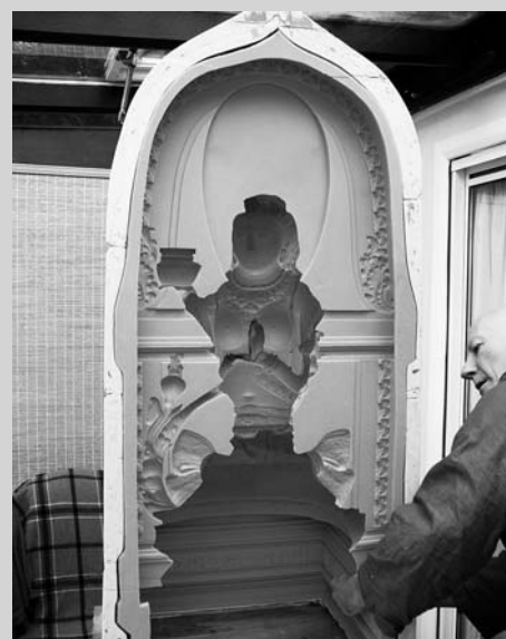
Ajahn Vimalo binds the hard plastic support mould to the soft rubber one. This casing is needed so the rubber mould doesn't lose its shape over time stretched by its own weight
